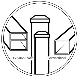
The Echelon Plus® post interior is reinforced
