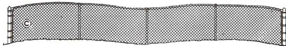
C Fence following grade
