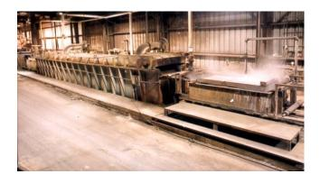
removing any impurities from the wire allowing a more secure bond between wire and coating. This provides a longer lasting product that continually resists peeling and corrosion while maintaining a new appearance year after year.
