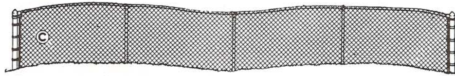
C Fence following grade
