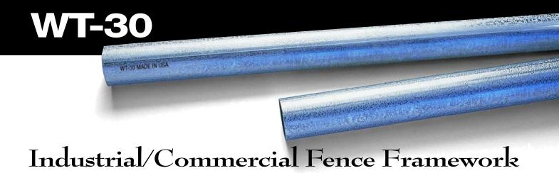
WT-30 is produced with high tensile/yield strength cold-formed steel. Wheatland's state of the art in-line ERW manufacturing process produces a uniform triple layer of O.D. protection against corrosion. The application of the highest quality zinc is followed by a convesion coating and top coated with brilliant UV clear polymeric coating for superior corrosion resistance.
